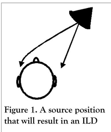
**Figure 1. A source position that will result in an ILD**
