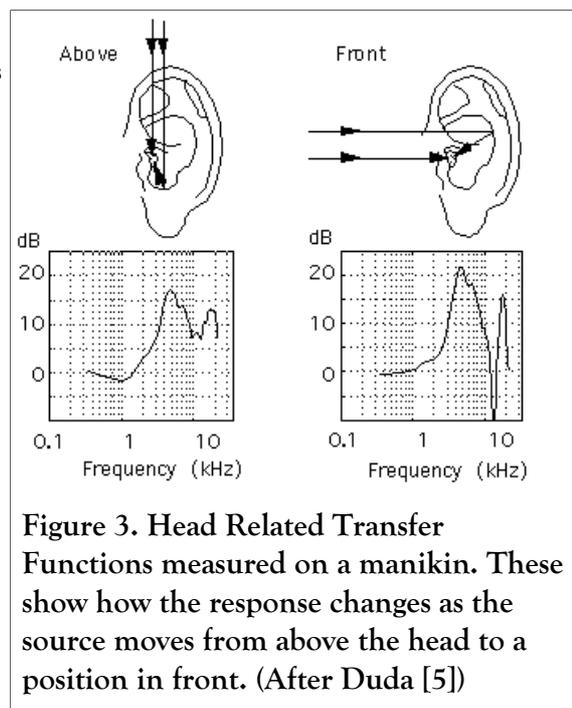
**Figure 3. Head Related Transfer Functions measured on a manikin. These show how the response changes as the source moves from above the head to a position in front. (After Duda [5])**
