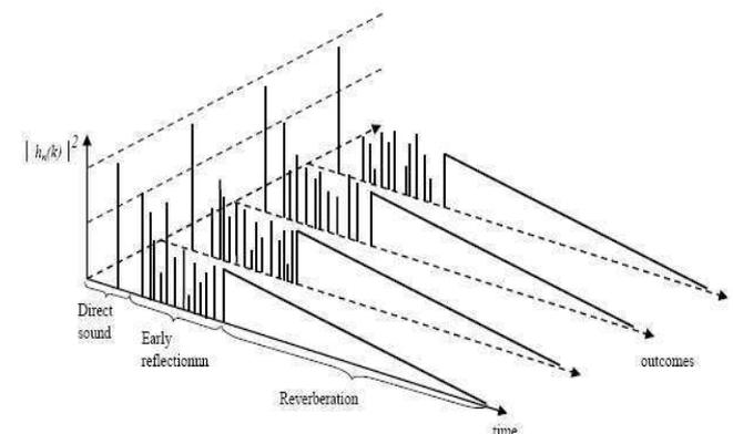
**Figure 3:** Examples of successive signals received by the microphone
