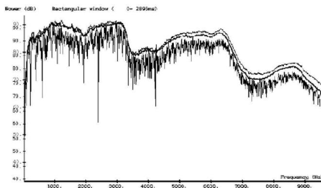
Figure 4. An example of how the proposed technique of coherent averaging an rotation of the source and microphone in a reverberant room can remove the reverberant sound component. Bottom trace is the stationary response, the middle trace is the rotated response and the top trace shows the anechoic chamber measurement of the response.
