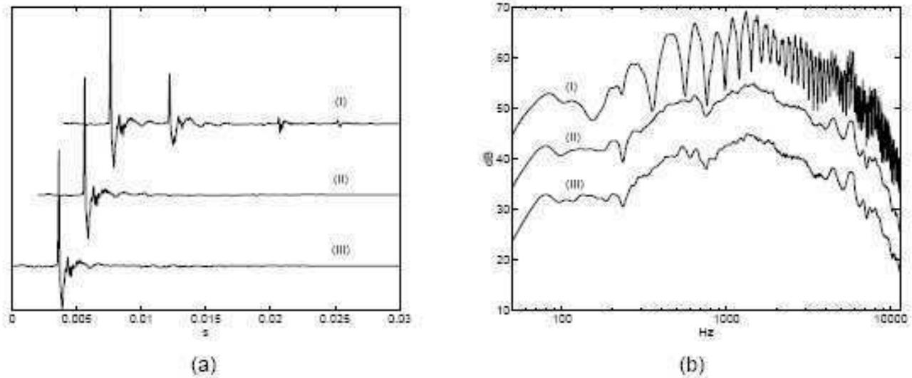
**Figure 2.** The responses of a loudspeaker found from MLS responses: (I) near a reflecting surface, (II) near a reflecting surface but with the loudspeaker and microphone rotating, and (III) in an anechoic chamber.
