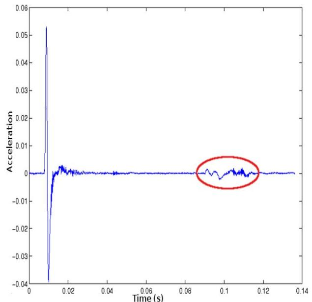
Figure 2. The low-pass filtered acceleration data as a function of time in seconds from the accelerometer on the Uni-Tapper hammer impacting on the ATC bare concrete floor. The acceleration associated with the hammer pickup is circled in red.
