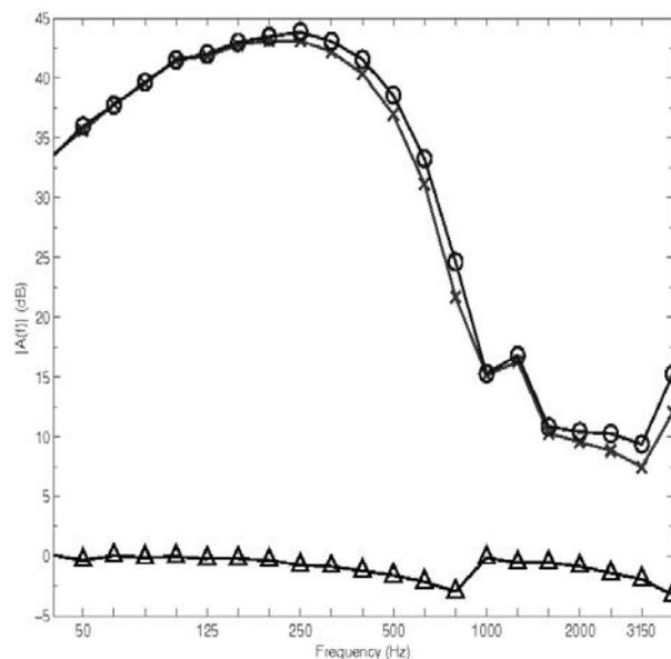
Figure 7: Acceleration spectrum levels with background noise, with a cork covering. With (x), and without (o), background noise, and the difference (◆).
