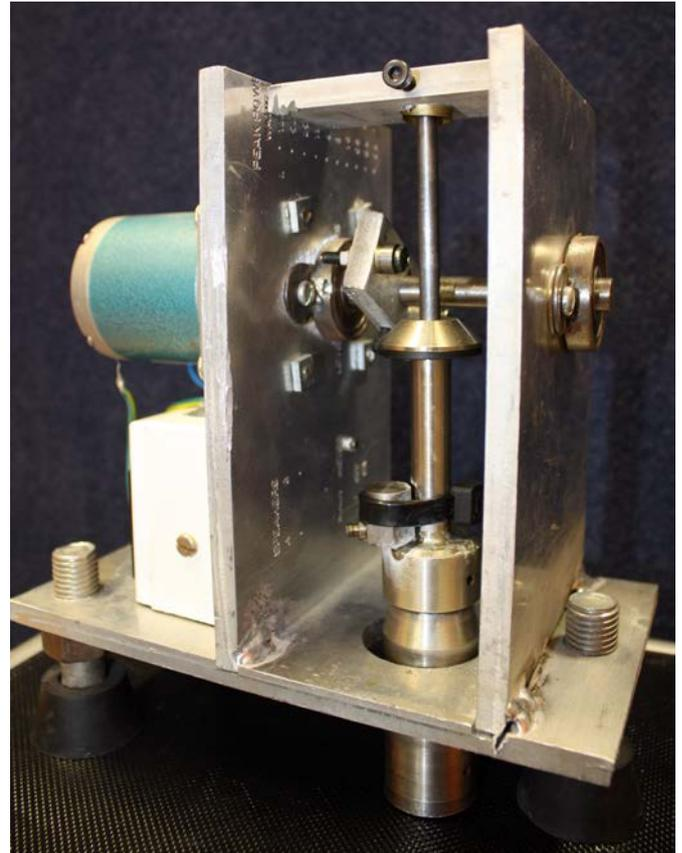
Figure 1. Uni-tapper with attached accelerometer.
