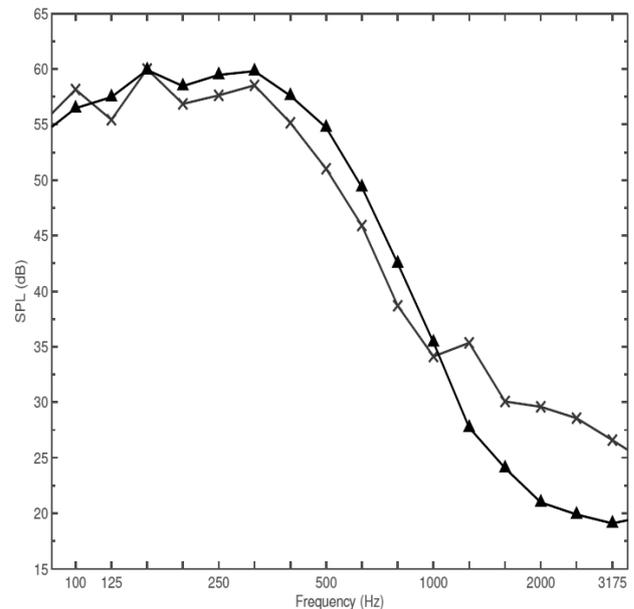
Figure 4. Normalised impact sound pressure level of the woodconcrete floor with a carpet floor covering, using only the acceleration spectrum of the hammer impacting the floor. Standard testing method (◆) and impulse response methods (x).
