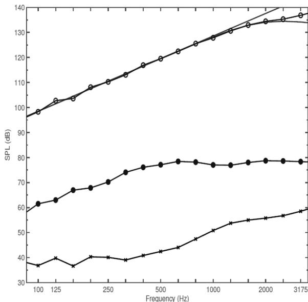
Figure 3. Verification of equation (7) to the measured  $L_n + R$ . Measured sound reduction index  $R$  (x) and  $L_n$  (●) and their sum  $L_n + R$  (○). Equation (10) is the straight red line and equation (7) is shown by the solid red line that begins to decrease to a -30dB/decade decline above 1900Hz.
