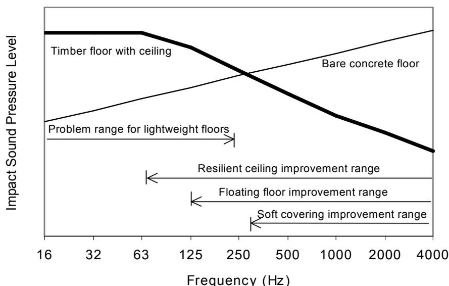
Figure 1. Impact sound insulation of a wooden floor compared to a concrete floor (after P. Sipari).
