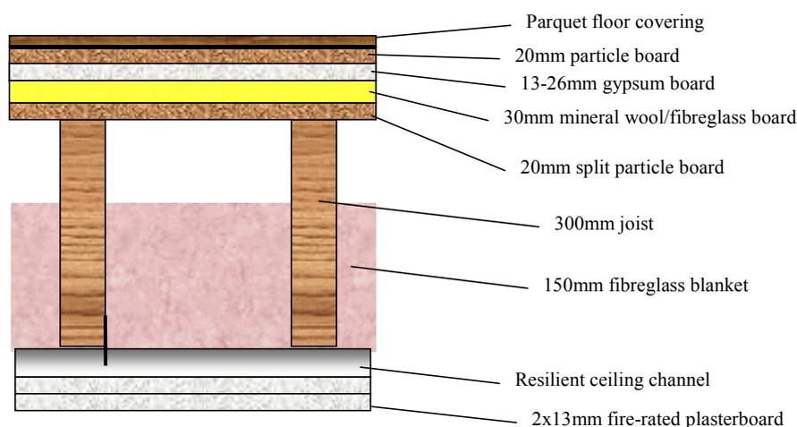
Figure 2. Generalised cross-section of floors used in pilot projects in Scandinavia. The floors used achieved IIC's of about 60–70dB.
