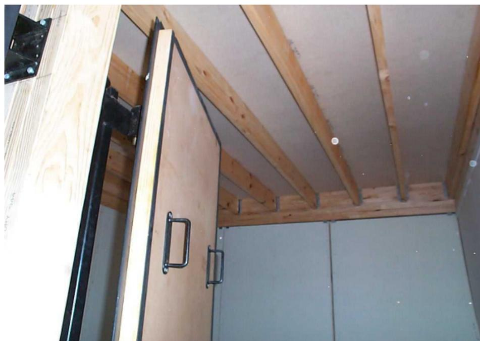
Figure 4. Inside the acoustic floor test chamber at the Forest Research labs. The view here is looking up at the beginnings of a simple floor, which at the time had no ceiling. The door shown is an inner door of a bivalve acoustic door system.
