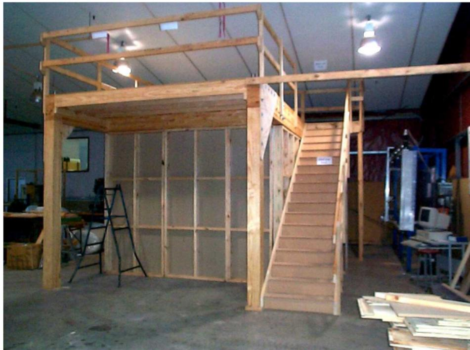
Figure 3. Exterior view of the facility for testing the impact insulation of floors at the Forest Research labs. The stairs lead up to the top of the floor. The floor frame and legs are made from glulam.
