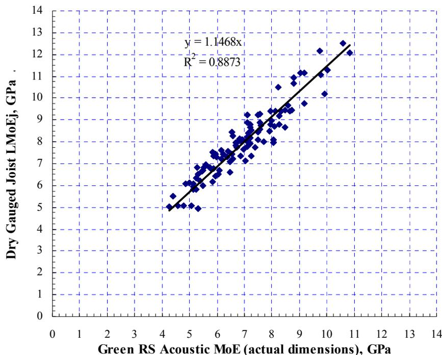
Figure 4: The relationship between acoustically measured stiffness of green timber and the stiffness of the same dry, dressed timber measured in a four-point bending test.
