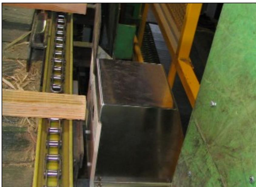
**Figure 3: The A-grader 'head' which strikes the end of the timber with a pneumatic hammer and listens to the response with a microphone.**
