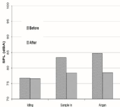
**Figure 12: Noise Levels Before and After Control at #2 Due to the Operation of the Three Other Mills**
