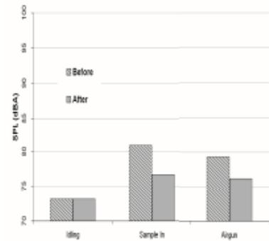
**Figure 10: Noise Levels Before and After Control at #1 Due to the Operation of Mill #2 Only**
