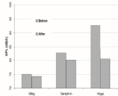
**Figure 11: Noise Levels Before and After Control at #2 Due to the Operation of Mill #2 Only**
