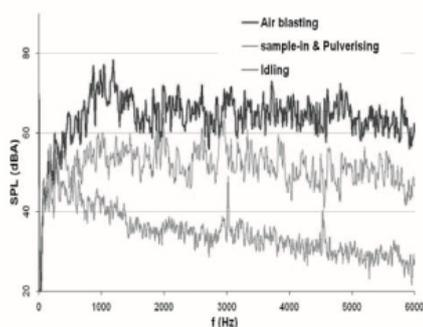
Figure 2: Noise Spectra at #2 When Mill 2# Operates Alone
