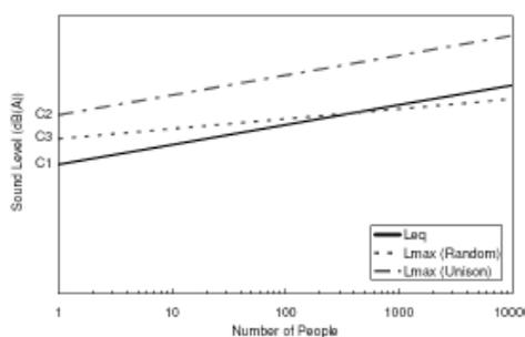
**Figure 3: Difference in the  $L_{max}$  noise level due to the crowd being random or in unison**
