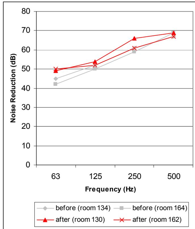
Figure 2: Measured Noise Reduction
