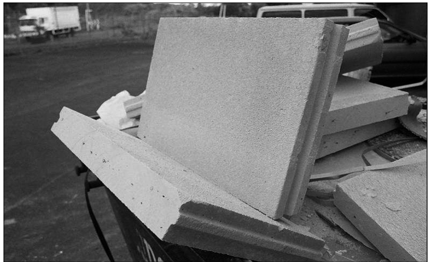
Figure 8 Aerated concrete panel used for the top layer.
