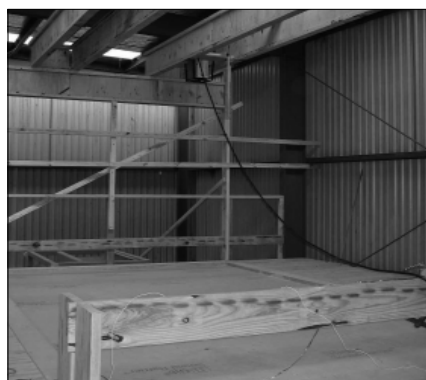
Figure 1: An electrodynamic shaker (left) and setups of the laser vibrometer to measure the floor (Centre) and Ceiling (Right)
