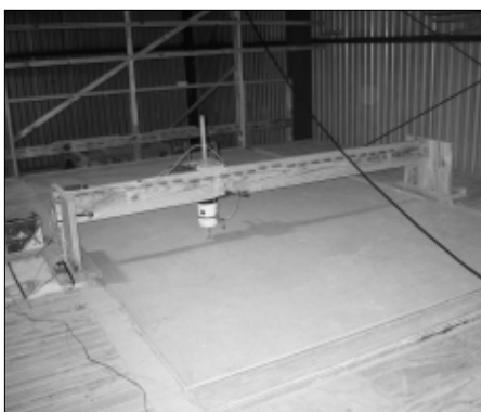
Figure 1: An electrodynamic shaker (left) and setups of the laser vibrometer to measure the floor (Centre) and Ceiling (Right)
