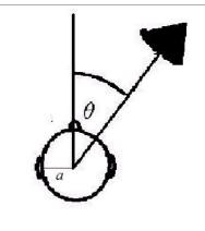
Figure 2. ITD depends on angle of incidence and head size
