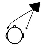
Figure 1. A source position that will result in an ILD
