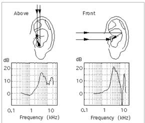
Figure 3. Head Related Transfer Functions measured on a manikin. These show how the response changes as the source moves from above the head to a position in front. (After Duda [5])
