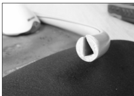
3.1.4. Plastic stripping approx. 12mm in diameter.
