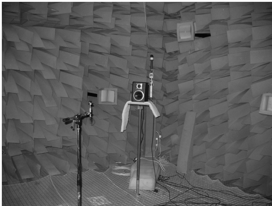
Figure 9: Anechoic room with a TetraMic A-format microphone array and Tapco loudspeaker response at a position within a room.
