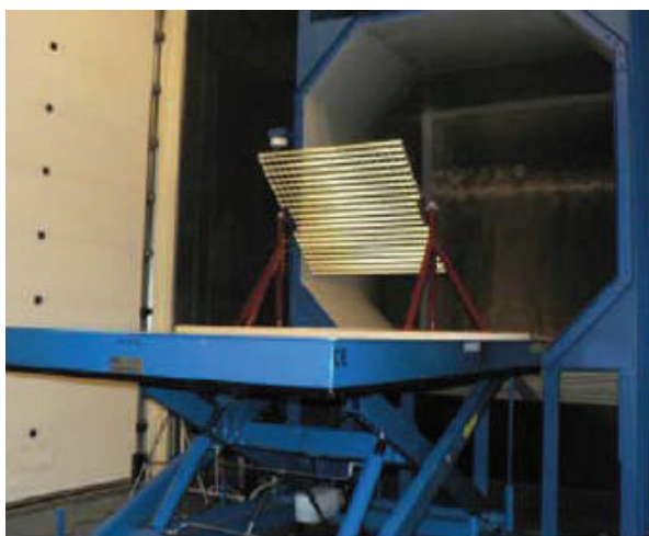
Figure 10: Wind tunnel test setup of façade element (left) and noise levels measured from test (right)
