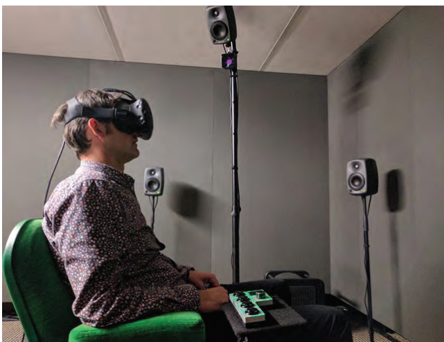
Figure 2: A person wearing the Vive VR headset in the loudspeaker array. The purple box under the loud-speaker in the top middle is a base station for tracking the position of the headset
