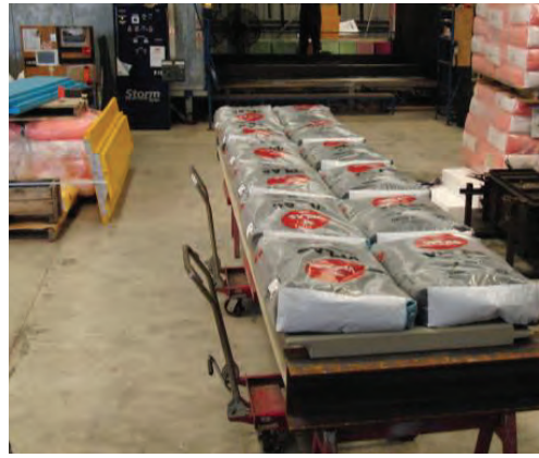
Figure 8: Load testing of a panel
