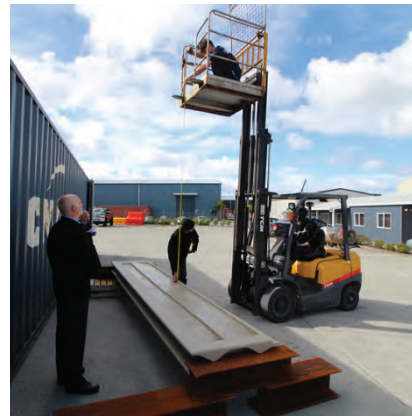
Figure 9: Impact testing of a panel from 3 m
