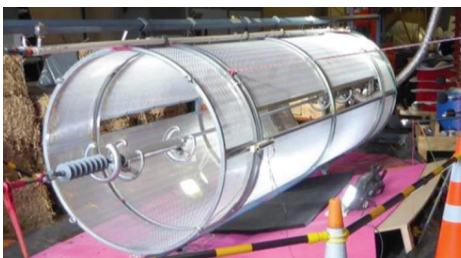
Figure 2: University of Canterbury corona cage
